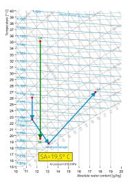
AdiabaticPro achieves in summer cooling mode temperature drops up to 15 K and stays under the supply air temperatures of conventional systems even at higher outside air temperatures.
